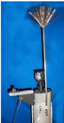
2. Dissipaters like the one pictured here don't work -- The problem with this approach is that the earth can supply a charge far faster than any set of discharge points can create ions. The earth can supply energy 4,000 times faster than the rate at which a static discharge brush can dissipate the energy!
